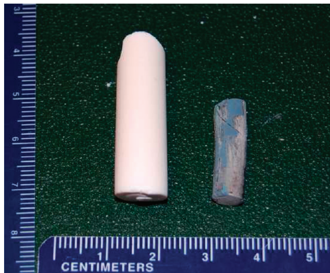
Figure 10. Photographs of a F-20-45 PAN-cross-linked silica aerogel monolith (left) and the resulting SiC aerogel monolith (right) after all processing steps (i.e., aromatization at 225 °C in air, carbothermal reduction at 1400 °C under flowing Ar, and oxidative removal of unreacted carbon at 600 °C in air).
